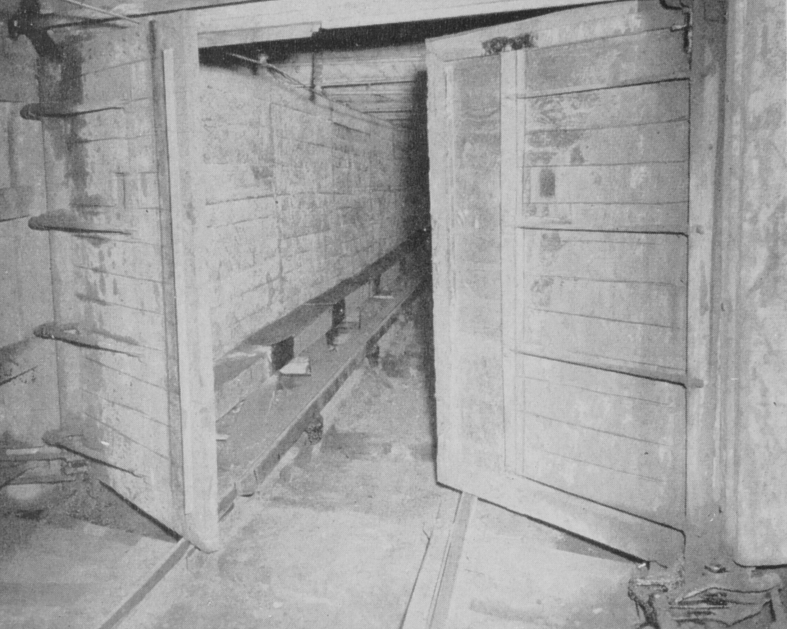
Automatically-controlled doors which regulate the flow of air in a mine.
