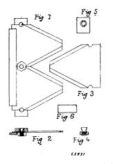
Edwin Roblin and John C. McCarthy, both of Belleville, Ontario, Canada, 24th April, 1899; 6 years. (Filed 21st January, 1899.) *Claim.*—In a reaper mower kuife, the back provided with countre-such holes with key slots to receive the key headed bolt, knife sec-tions with key slots to receive the key headed bolt, knife sections with half circles on adjacent sides for the passage of the fasten-
