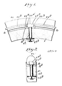
shoulders  $a^3$ , to engage the channel piece at the edges of the opening  $b^2$ , the rigid horizontal shoulders  $a^4$ , and the locking bolt d, co-operating with said shoulders  $a^4$ , substantially as described.
