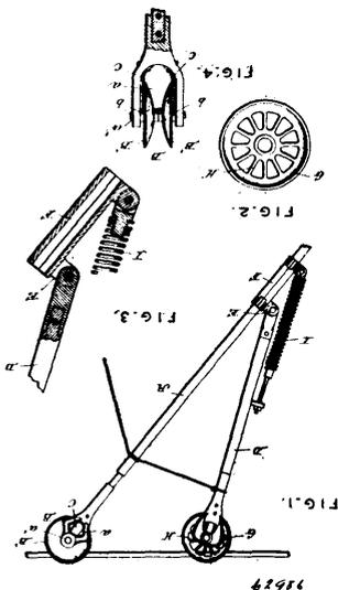
having ribs, said ice-clearing wheel being formed in two parts, and a spring bearing against the short pole to hold it yieldingly in contact with the wire.
