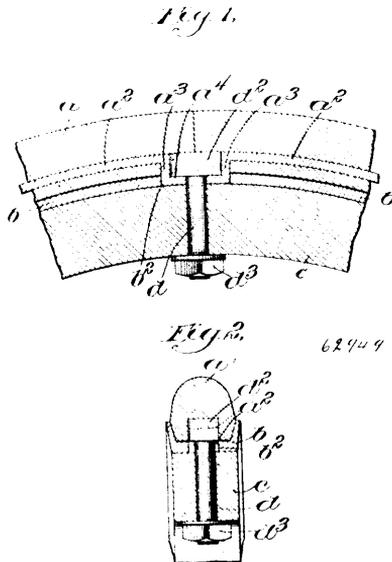
shoulders *a*<sup>3</sup>, to engage the channel piece at the edges of the opening *b*<sup>2</sup>, the rigid horizontal shoulders *a*<sup>4</sup>, and the locking bolt *d*, co-operating with said shoulders *a*<sup>4</sup>, substantially as described.
