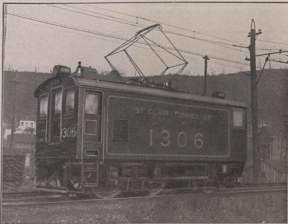
G. T. R. single phase locomotive for passenger and freight service in St. Clair Tunnel.
