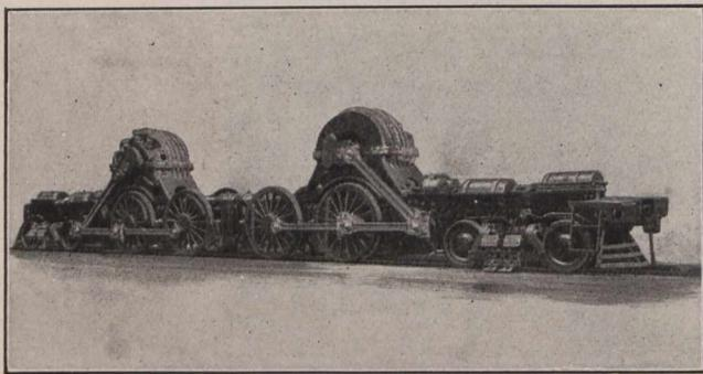
**Pennsylvania double articulator locomotive for New York tunnel service—View of under frame, motors and driving mechanism.**
