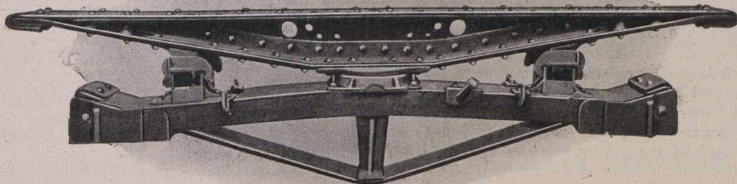
Simplex Body and Truck Bolster and Susemihl Side Bearings.
