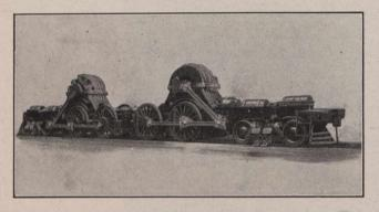
Pennsylvania double articulator locomotive for New York tunnel service—View of under frame, motors and driving mechanism.
