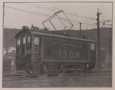
C. T. R. single phase locomotive for passenger and freight service in St. Clair Tunnel.
