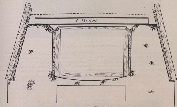
Fig. 6. Flat Top Culvert.
