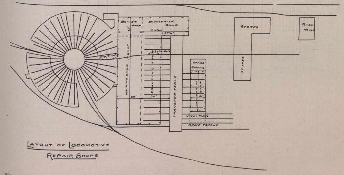
wires and trolleys erected at one side of the transfer table pit. The motor is also connected by means of clutches, to a winding drum which carries a steel cable, used for moving the engines from their respective pits, to the lifting jacks near the centre of erecting shop, and by using a snatch block arrangement they can be moved back into the shop as required.
