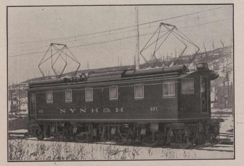
New York, New Haven and Hartford direct current railroad, simple phase in locomotive for freight and passenger service, spur geared motors and placed directly over driving axles.
