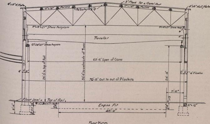
Section. of Erecting Shop
