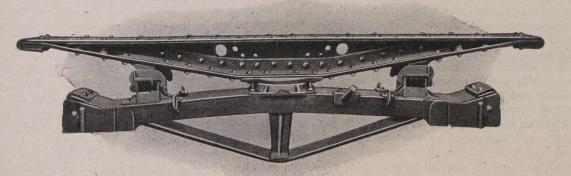
Simplex Body and Truck Bolster and Susemihl Side Bearings.
