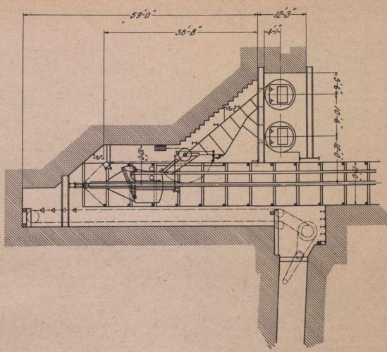
Plan C-Dominion No. 2 Colliery. Sketch of the Hoisting arrangements on the Phalen Seam, showing Tipples, Storage Chutes, Hoisting Tank, and Guide Spears
