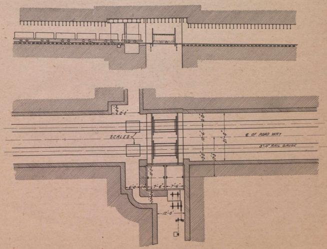
Plan B-Plan and Elevation of Dominion No. 2 (Phalen) Pit Bottom
