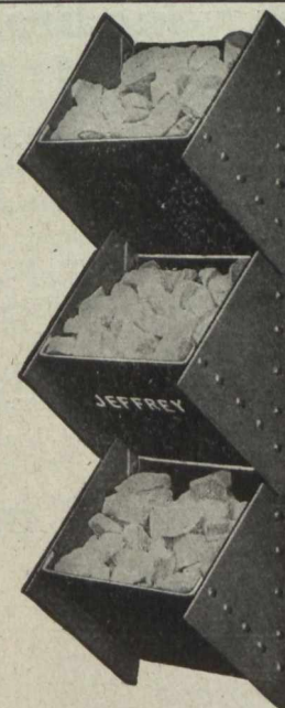
"Continuous Flanged Back" Elevator Buckets For handling crushed stone. The flanges of bucket serve as sides to a discharge chute to the bucket following.
