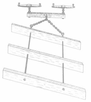
degrees, as shown in the accompanying sketch, on the front and bottom edge of the deal affix an iron platesay about two inches wide by 1-inch thick-allowing it to project about 4-inch below the deal (abandoned or half-worn sled shoes will serve this purpose well); then floor over the frame in part with inch boards, making convenient standing room for the teamster while in
