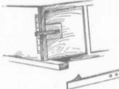
with a catch at the end and fastened to the side of the cart, as shown, is exceedingly simple, effective and convenient. A slight tap with a good stick and the tail board is released. The latter has an iron strap along the end to keep the board from splitting by equalizing the pressure.
