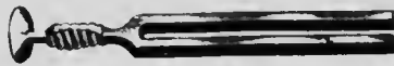
Gardiner Brown's tuning-fork: middle C, of 512 vibrations per second (one-third natural size).
