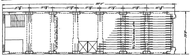
Typical Floor Plan, Mason & Risch Liano Warehouse, Toronto. Showing the Spacing of Beams, Columns and Lloor Steel, Together With the Length and Width of the Building. Bond & Smith. Architects.
