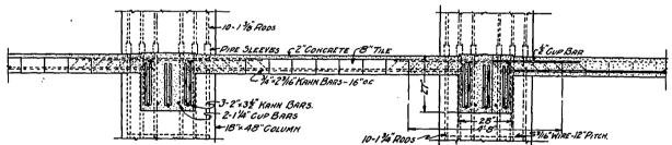
Longitudinal Section of Typical Floor, ason & Risch Plano Warchouse, Toronto. Showing Location of Columns and Disposition of Steel Bars. Although the Columns are Approximately 14-Foot Centres, Making the Floor Panel 14x25 Ft.. it Will be Noted that the Total Thickness of Hollow Tiles and Concrete Joists is Only 10 Inches. Bond & Smith, Architects.
