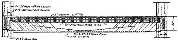
Transverse Section of Typical Floor, Mason & Risch Piano Warehouse, Toronto. Showing Alternating Arrangement of Hollow Tlie and Concrete Joists, Together with Typical Floor Beam, 25-Foot Span, Reinforced with Kahn Bare. Note the Narrow Width of Column. Bond & Smith, Architects.
