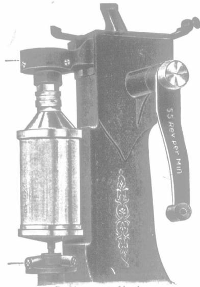
The Magnet Cream Separator is the exception and it is made by us. It has a bowl supported at the top as well as the bottom. Examine the accompanying cut and you will see how nicely the bowl of the Magnet is held in its place, giving it steadiness of motion and preventing it getting out of balance. It also makes it very easy to turn, in fact so easy that a child of four years can operate it. See page 18 in our catalogue.
