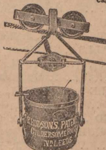
61—Rope Bucket, with R. H.'s Patent Catch for Wire Rope Trucks
