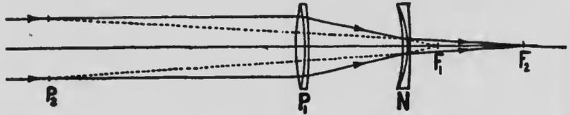
FIG. 45. Telephoto Lens.
