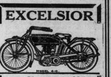
1 ... Mo\_e. Uniy \$250 It is our chain-drive single and is the only motorycle selling at this price you can get equipped with Borsch Armored Magneto, also with a clutch operated by simply turning left grip, making it unnecessary to take hands off your bars; and we supply a carrier, also foot rests, without extra charge.
