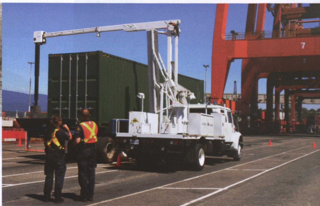
Terrorist groups could use container shipping to deploy WMD. The Canadian Border Services Agency uses a mobile vehicle and cargo inspection system to detect weapons and other dangerous goods in marine containers.
