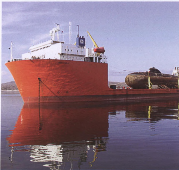
A decommissioned nuclear-powered submarine is loaded onto a heavy-load transport vessel and brought to the shipyard to be defuelled and dismantled.
