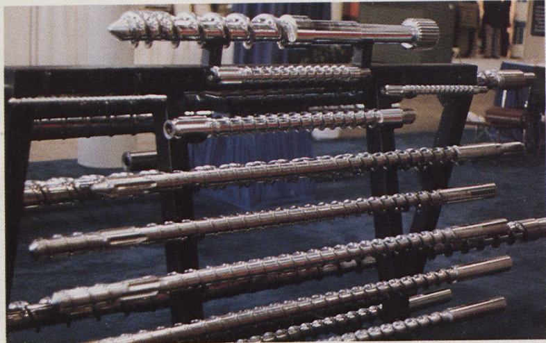
North America's largest feed screw manufacturer, Canadian Feed Screws, produces extruder screws and barrels for the plastic, rubber and food processing industries.
