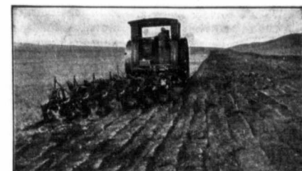
Avery 40-80 H.P. "Light-Weight" Tractor and 8-bottom Avery "Self-Lift" Plow doing breaking.
