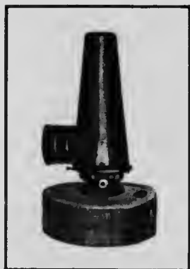
Fig. 19.—An egg tester. The egg is held in front of the opening in the short tube to the left which is directly opposite the flame in the lamp.
