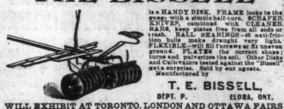
is a HANDY DISK. FRAME locks to the gang- with a simple half-turn. SCRAPER KNIVES, combined with CLEANER BARS, keep plates free from all sods or trash. BAIL BEARINGS-40 anti-friction balls make draught very light. FLKXIBLE-will fill furrewes fit uneven ground. PLATES the correct shape; turns and pulverizes the soil. Other Disks and Cultivators tested against the "Bissell" gets surprise. Sold by our agents.
