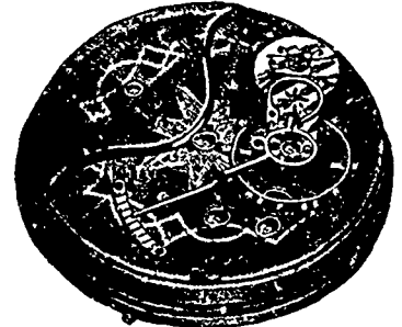
18 Size, Nickel.—No. 27, Hunting, or No. 97, Open Face, pendant set, 16 jewels, adjusted, extra centre jewels, Breguet hair spring, patent regulator, double sunk dial, jewels set in red gold settings.
