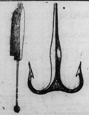
This cut represents the Norwegian Jigger, which is one of the greatest fish killers in the world, and used exclusively in Norway. Can be had from all the Hard-ware Store in St. John's. Remember it is important to With the exception of about a score, use two swivels in order to make the Jigger spin.
