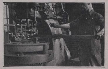
Car Wheel Borer Lift Hook Attached to Air Hoist.
