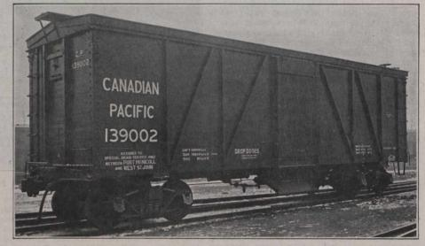
Hopper Bottom Grain and Coal Car for C.P.R.
