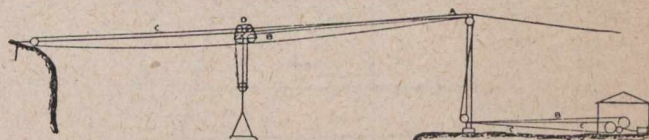
FIG. 21—Horizontal cable hoisting plant
