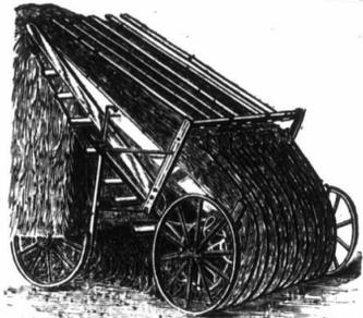
The above cut shows the Foust's Hay Loader with Anderson's Patent Rake Attachment. It will take up grain with short straw. It will take up grain as clean out of the furrow as on the ridge, without the necessity of using the horse rake. In hay it can be used after the Tedder, and will take it from the swarth without using a horse rake.
