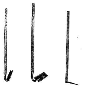
Fig. 3-Draw-scoop Fig 4-Broadscoop Fig. 5-Pipe-layer
