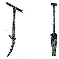
Fig. 1.—Tramp-piek. Fig. 2. -Semi-cylindrical spade.
