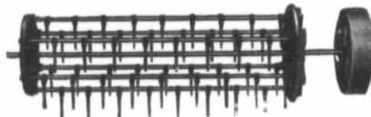
This is the separating device that does such wonderful work in tearing up the bunches and spreading out the straw that it enabled Avery Separators to make a record of 99.9-10 per cent of the grain saved in 27 canvas field tests—the best proven grain saving record ever made.
