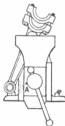
Fig. 2—The right way to clamp a connecting rod in vise.
