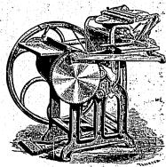
These Presses are all built with the latest improvements. and of the lutest style introduced by the Inventor. In the Quarto and Half Medium, in combination with the Ink Distributing Table above the form, are used a Oplinder, a Vibrating Feed Rolley; and a Fountain, below, the form.
