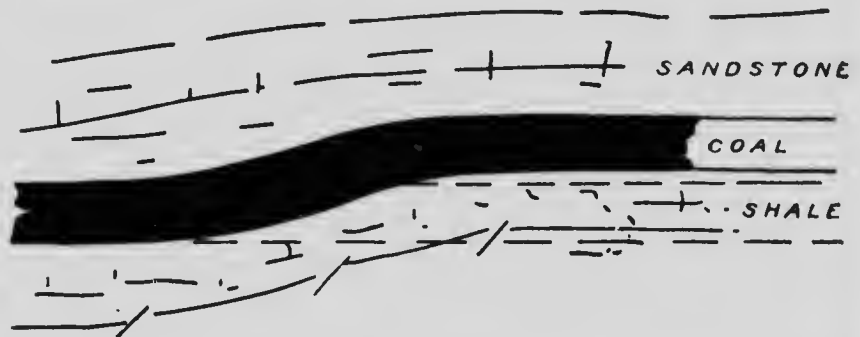
Fig. 15. Diagram illustrating the wave-like effect produced by subsidence, as distinct from the step-like effect of faulting. Wherever each layer about a seam has great adherence this wave-like change occurs.
