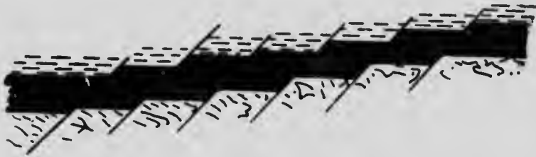
Fig. 16. Exaggerated effect on strata which is blocky: indicating successive advances of the face, and showing fault-like results. Most destructive shattering of roof and coal.
