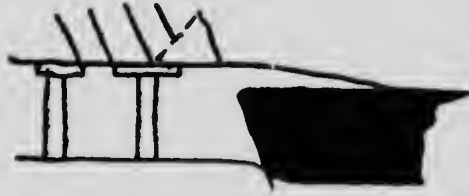
Fig. 23. An effect in an upper seam caused by operating a lower coal.
