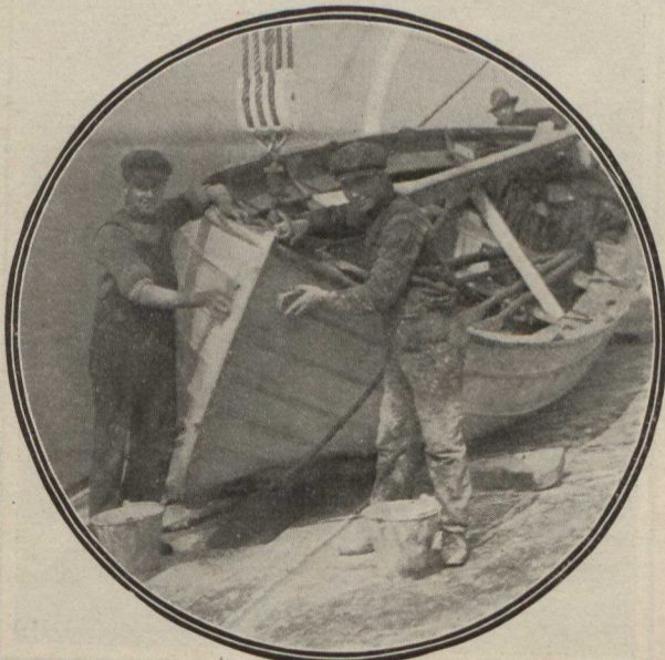
Life-boats are Always Carefully Overhauled, Scrubbed With "Sougee" and Painted.
