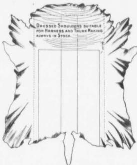
Sadler & Haworth's Diagram of Hide showing the part used for the manufacture of our Belting.
