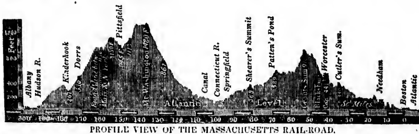
PROFILE VIEW OF THE MASSACHUSETTS RAIL-ROAD.
