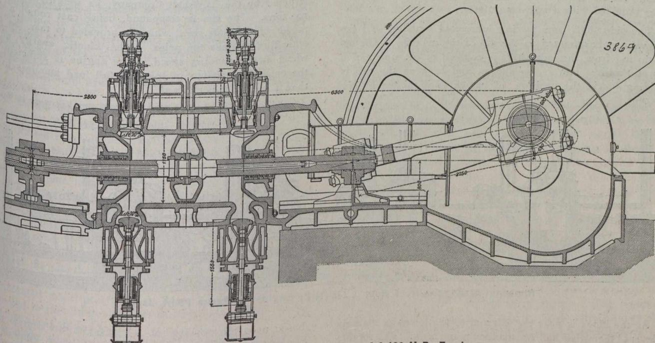
**Details of Cylinder and Valves of 2,130 H.P. Engine.**
