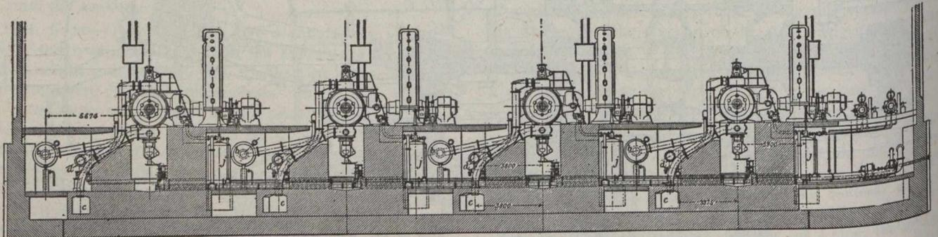
Showing Arrangement of Four 2,130 H.P. Engines in Power Plant, Japan.
