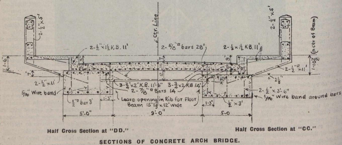
NOTE:—Designed for live load of 125 lbs. per sq. ft., or 10 and 6 tons at 10-ft. centres on roadway and 100 lbs. per sq. ft. of sidewalk. All concrete 1:2:4. Where joints have to be made set forms square with surface with steel projecting through. Joints in beams and slabs to be at centre of span.
