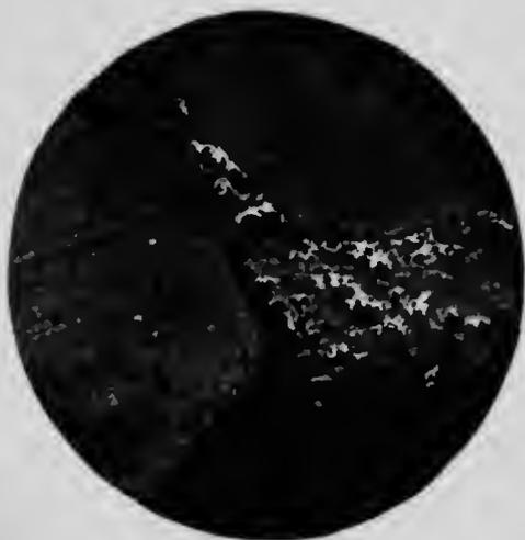
Chalcopyrite cutting Pyrite (blued) and Pyrrhotite (black).
