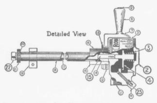
The minimum burner flame Pilot and the Independent Pilot must be properly adjusted by the person installing the Range.
