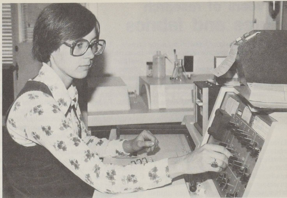
NRC's Dr. Roxanne Deslauriers sits at a smaller so-called "low field" NMR spectrometer. She is developing methods to study metabolism, the integrated web of chemical events that characterize life. (Photo: Bruce Kane, NRC)
