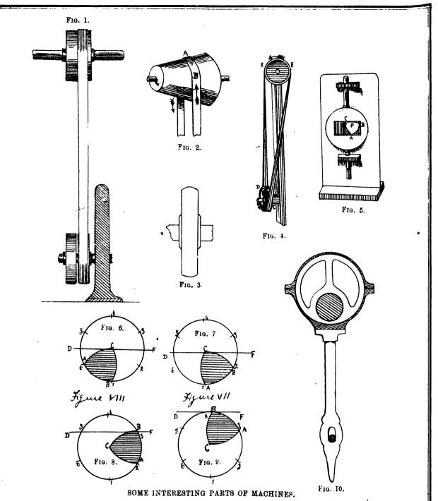
To consider the motion preduced, let us take, instead of the sketch of the machine itself, the four following figures; where the shaded portion represents the cam in four different positions it will pass through during a half revolution. The path of the side A B, opposite to the centre C, is also shewn by a circle divided into six equal parts, in the points 1 2 3 4 5 6, so that, by the principles of geometery, A B must be equal in length to any one of these parts.
