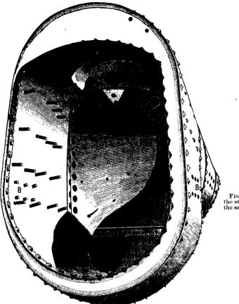
F19.3.—Cross section of the body and the patch, showing the screw stay-bolts; the upper one of the left-hand row being the same as D, Fig. 2.
