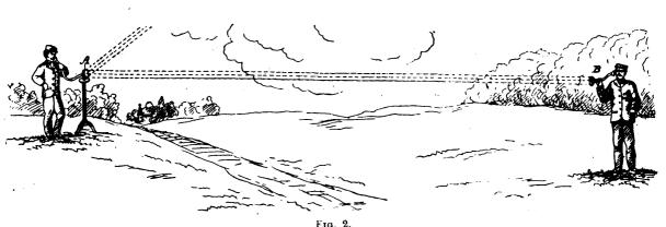
the lampblack cell is connected with a telephone and galvanic battery, and exposed to the influence of an intermittent beam of of sunlight, a loud musical tone is produced by the telephone. This result seems to to be due rather to the physical condition than to the nature of the conducting material employed, as metals in a spongy condition produce similar effects. For
