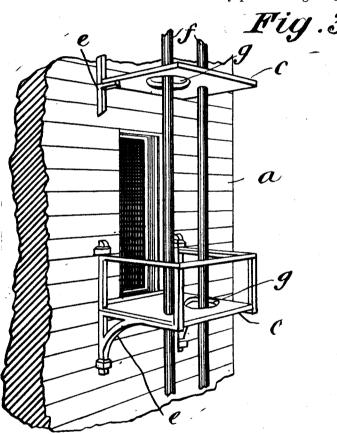
floors or staging from the roof to the ground; g g are circular openings which alternate from one side to the other at each succeeding landing. The landing to be placed before a window at every story.
