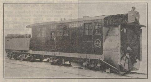
Fig. 26. Leslie Bros. Rotary Snow Plough, with Ice Cutters and Flangers.
