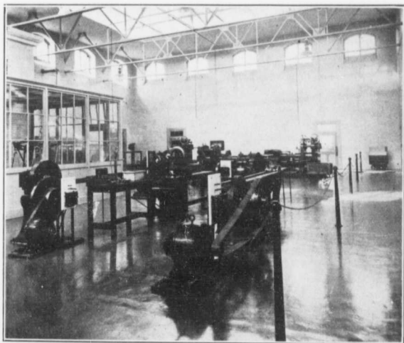
Fig. 12—General view of Rolling and Adjusting Room, showing draw-bench, automatic trying cutter, and scale room.
