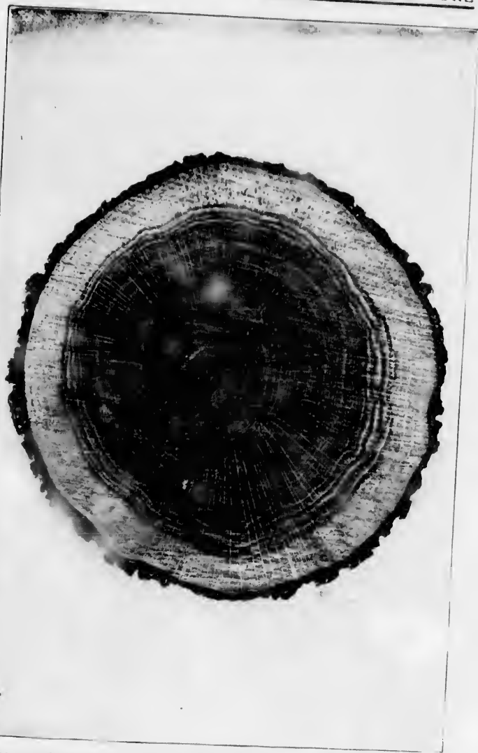
Transverse Section of Trunk of White Oak, Quercus alba , Showing BARK, Sapwood, Heartwood, Annual Rings and Medullary Rays.
