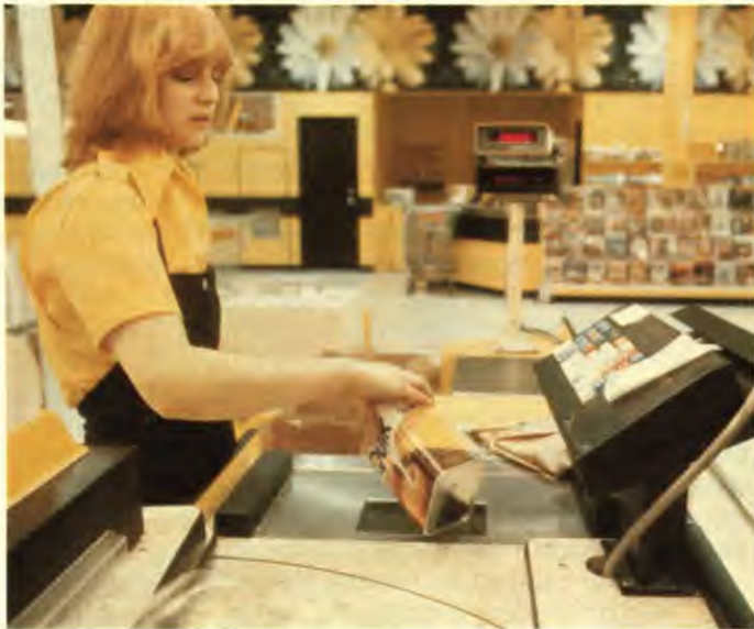
Many Canadian supermarkets, such as Steinberg's, have introduced computerized check-out counters which can automatically identify the "universal product code" now found on much merchandise.
