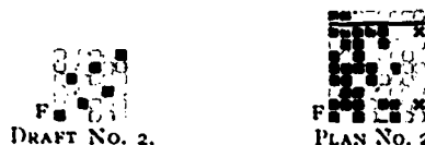
Weaving, 1 pick face weft 1 " back " X 1 " face " 3 picks repeated. 57 picks per inch.
