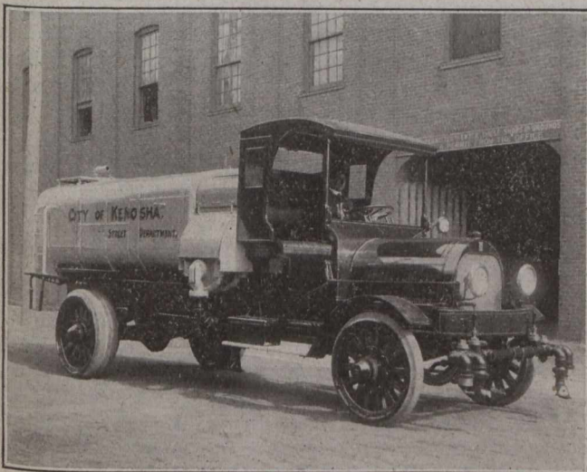
Fig. 7.—Two-Motor System Combination Power Flusher and Sprinkler, Complete with Electric Lighting and Starting Equipment; 1,200-gallon Tank.
