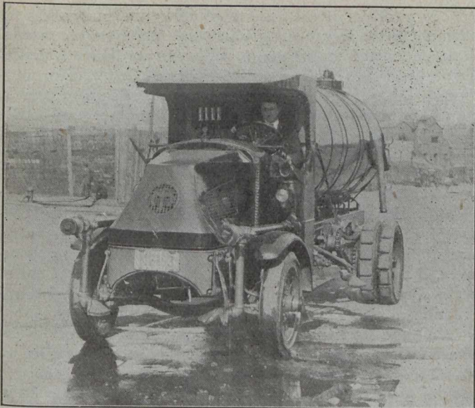
Fig. 5.—Auto Flusher. Note Fixed Nozzles and Sprinkler Heads.
