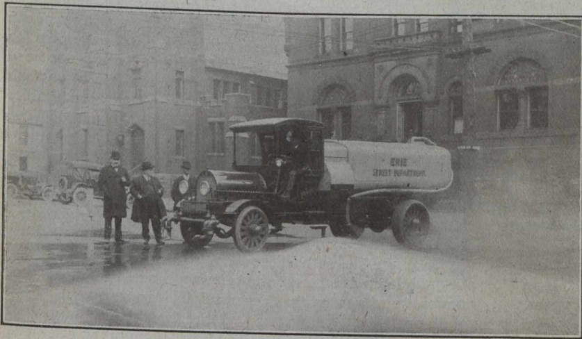
Fig. 1.—Two-Motor System Combination Power Flusher and Sprinkler.
