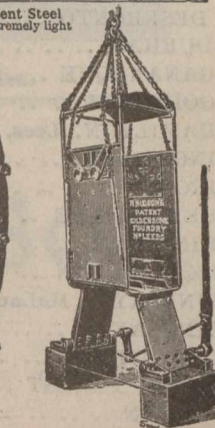
15—R. H.'s Improved Steel Cage, with Safety Grippers and Fallers complete
