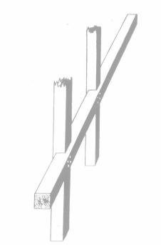
Fig. 2.-Showing a Rack-lifter Girt, with Projection on Which the Sill of the Lifter May be Slid Past the Posts.
