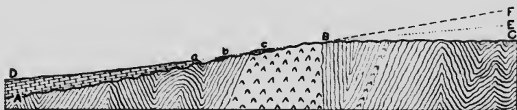
FIGURE 1.—AB represents the plain beneath the sedimentary cover; BC, the plain north of the edge of the cover; DB, the plain over the surface of the sediments; a, the escarpment, b and c, outliers. Vertical exaggeration about forty times.
