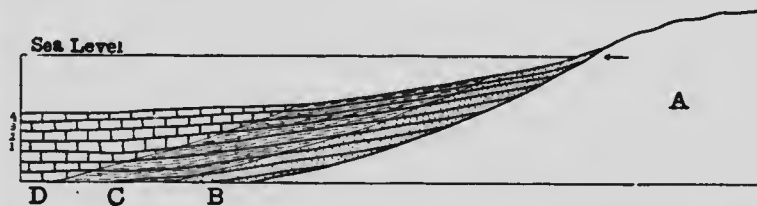
FIGURE 9.—Diagram to represent the normal distribution of sediments. A, oldland; B, sandstone and conglomerate zone; C, shale zone; D, limestone zone. Transition zones are indicated by lines.
