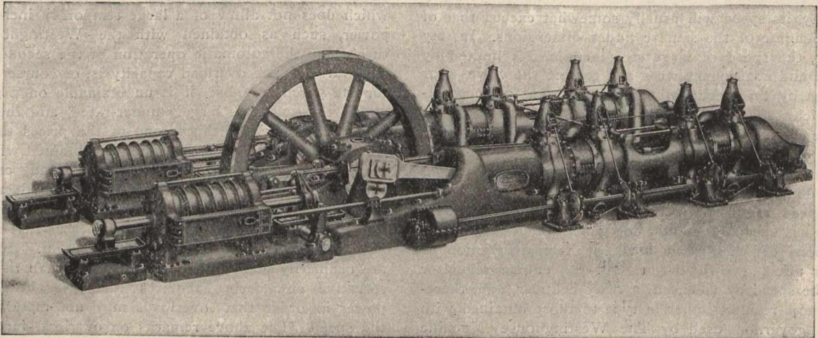
Westinghouse Gas Driven Blowing Engine for Blast Furnace Gas. Heavy Duty Twin Tandem Type.
