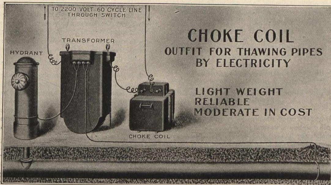
used in connection with the primaries of a standard transformer and one for lighter service, consisting of a transformer adapted for suitable secondary voltage adjustments, mounted in cast-iron top and bottom frames, and intended to be used directly on the primary mains. The connections are simple and easily made, and the operator is entirely protected from injury.
