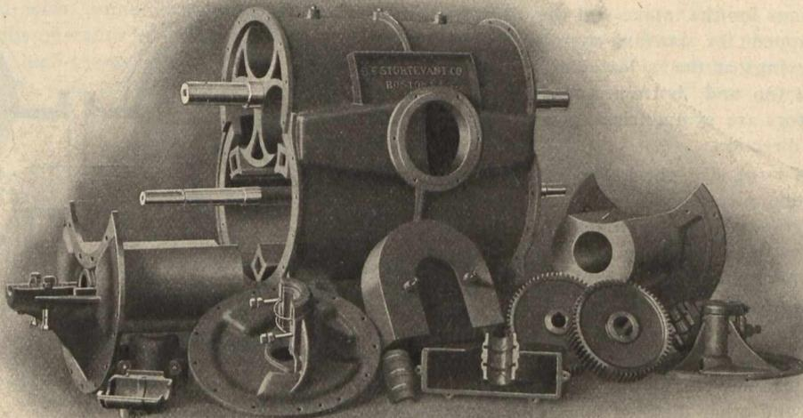
Fig. 6.—Parts of High Pressure Blower.
