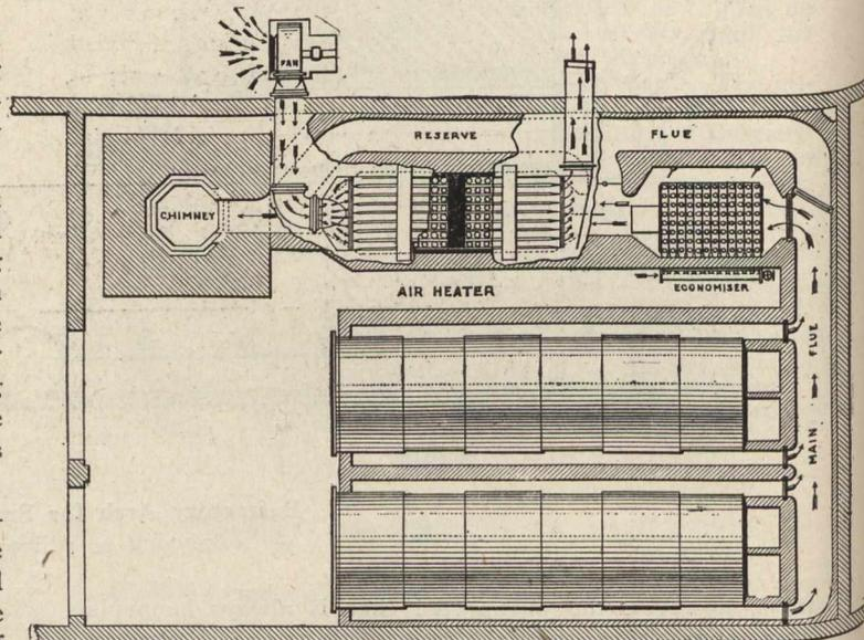
Fig. 3. Combined Installation of Heater and Economizer.
