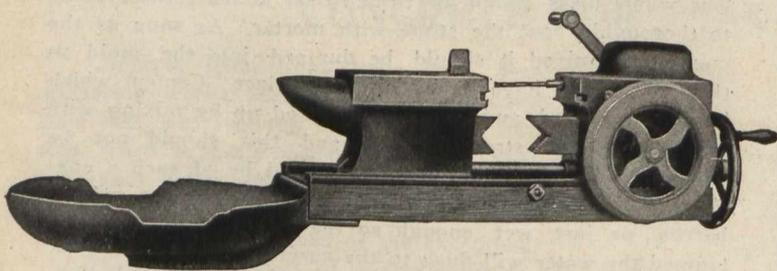
Detroit, Mich., are to be congratulated on their new product. The device consists of a steel-faced bed, or base; at one end is a stationary head stock, at the other a moveable tail stock and an overhung forge pan. The head stock contains the mechanism of the rotary blower, drill-grinder, and the
