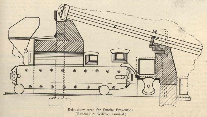
It is, however, the unexpected that is always happening. This month, through the courtesy of the above mentioned company, we have pleasure in setting before our readers a new arrangement of furnace and stoker recently introduced in connection with their boilers, which it is claimed "is absolutely smokeless, even when running 50 per cent. overload."\*
