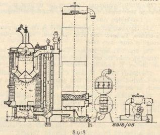
the refractory walls. This result is secured by the arrangement between the retort and the shaft of a central cone together with an inverted conic frustrum, the central cone being provided with suction passages which abut on the refractory material of the shaft, whereby the suction of the gas is caused to take place inside the central cone only.
