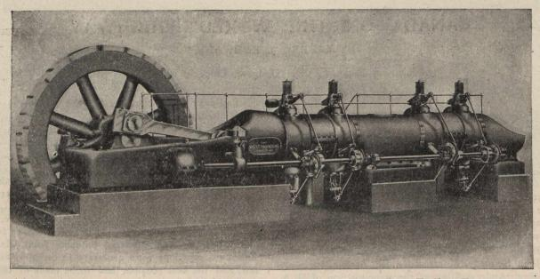
Westinghouse Horizontal Double Acting Gas Engine. Heavy Duty Tandem Type.
