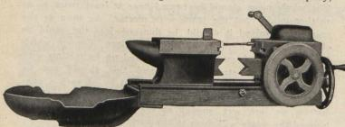
Detroit, Mich., are to be congratulated on their new product. The device consists of a steel-faced bed, or base; at one end is a stationary head stock, at the other a moveable tail stock and an overhung forge pan. The head stock contains the mechanism of the rotary blower, drill-grinder, and the
