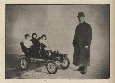
has two speeds forward, and one reverse, power being transmitted to the rear axle by a Cardan-shaft. The tonneau is detachable, has two side-doors, and accommodates four passengers as shown in the picture. All levers and pedals necessary for a perfect control are provided, also two brakes and five lamps. As will be noted, a baby-chauffeur has been trained to run the automobile, which is the smallest working model ever produced, weighing only 243 pounds.
