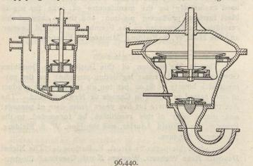
chamber along with the current of air whereby it is carried will be absorbed or precipitated by the liquid, and the liquid thus charged with dust will be caused to pass along with the air through the pump.
