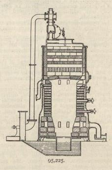
non-return valves on the air inlets; also having an improved steam-raising and heat-storing device consisting of metal and brick checker work placed upon the incandescent zone at the top of the gas producer, and combined with a suitable water supply.
