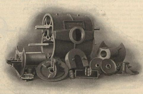
Fig. 6.—Parts of High Pressure Blower.
