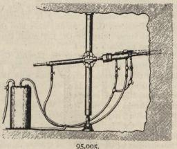
nected to an atomizer attached to the drill cylinder, from which atomized jets of water are discharged around the edge of the hole being drilled, thus laying all dust arising therefrom. Gas Producer Generator.—H. G. Hills.—95,225.—The invention consists of a gas producer arranged to have an upward draught-blowing period, alternating with the downward passage of steam during the gas-making period and
