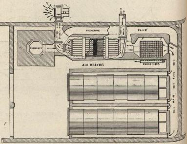
Fig. 3. Combined Installation of Heater and Economizer.
