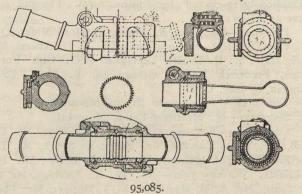
each having projecting lugs and wings on their sides, which are interlocked by partial rotation upon a horizontal transverse axis, suitable spring-actuated locking and releasing devices being arranged in conjunction with the interlocked portions.
