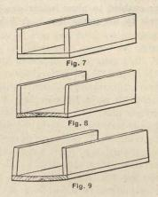
thicknesses. A pattern like Fig. 7 is more serviceable made with length of the bottom piece running from one rib to the other, as the bottom will stay straight and the side will always draw. If made like Figs. 8 and 9 you get the effect shown which will distort the ribs so that the pattern will not draw.
