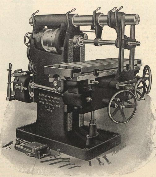
Plain Milling Machine. Gear feed. Double back gears. Range 46 x 14 x 20 ins.
