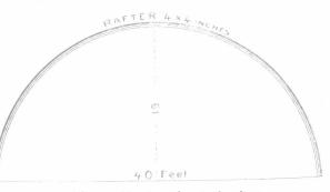
Fig. 2.-Semicircular-roof rafter.
